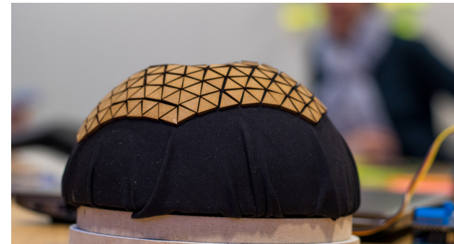
Figure 14. Half a dome with a servo motor inside, that pushes through the fabric to mimic a kick of a baby. The MDF triangles are used to create a visually appealing look.
